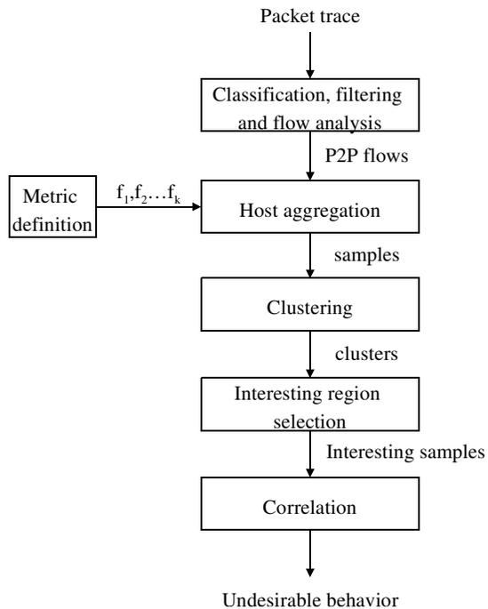
Figure 1: Schematic overview of the proposed methodology.
