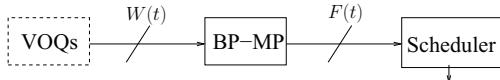
Fig. 2. Assisted scheduling approach: BP-MP module feeds the scheduler with the BP-messages instead of the queue lengths.
