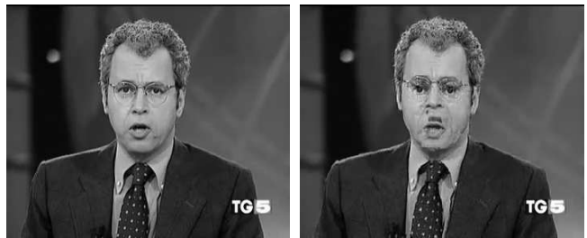
Fig. 5. A frame of video ‘television news’: original frame (left); decoded at the receiver side when configuration 1 is used and some packet losses occur (right)
